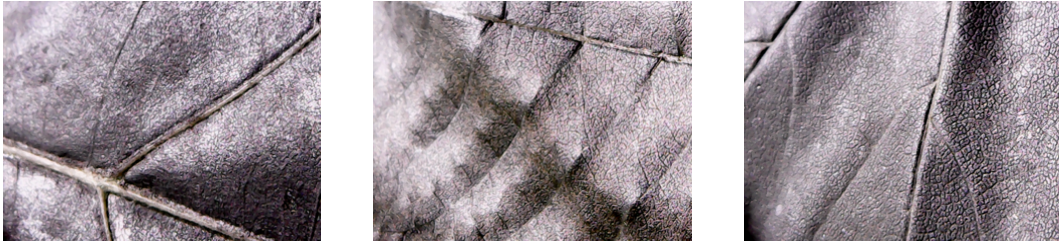
Figure 7.1: From left to right: Red Oak, American Ash, and Sugar Maple through H polarization filter in the Specular Direction.
